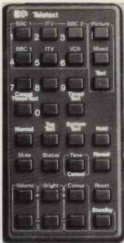
A Pye push-button Teletext remote controller. It is an ordinary TV controller with a decimal keypad.
